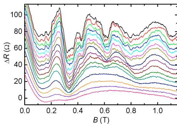
**FIGURE 2.** TMF spectra of the 1.2  $\mu\text{m}$  InSb sample with linear background subtracted. From top to bottom,  $T = 4.5, 6, 8, 10, 13, 16, 20, 25, 30, 40, 50, 60, 80, 100, 125,$  and 150 K. Traces are offset by 5  $\Omega$ . The split maxima merge at  $\sim 80$  K, at lower  $T$  than the TMF maxima smoothing out at  $\sim 150$  K.
