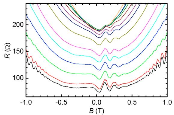
**FIGURE 3.** TMF spectra of the 2.0  $\mu\text{m}$  InAs sample. From top to bottom,  $T = 60, 50, 45, 40, 35, 30, 25, 20, 15, 12.5, 10, 7.5, 5,$  and 4 K. The split maxima merge at  $\sim 20$  K, at lower  $T$  than the TMF maxima smoothing out at  $\sim 60$  K.
