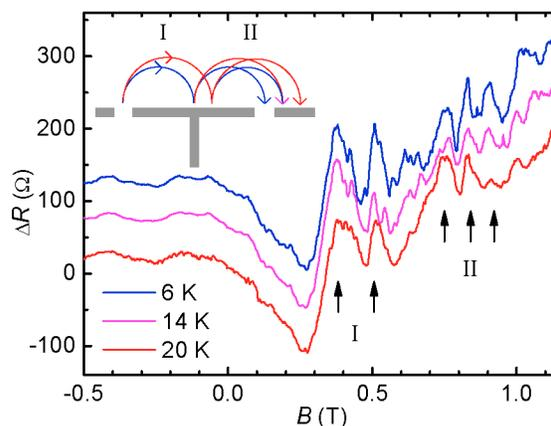
**FIGURE 1.** TMF spectra of the  $0.6$   $\mu\text{m}$  InSb sample show doublet and triplet structures for the first and second focusing maxima, respectively. Traces are offset by  $50$   $\Omega$ . Inset: Schematic plot of the focusing structure and spin-split ballistic trajectories.
