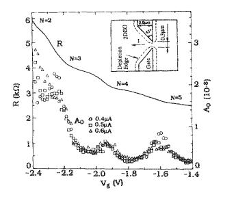
FIG. 1. R vs  $V_g$  and  $A_0$  vs  $V_{g'} A_0$  is obtained by fitting  $S_i = A_0 I^2 / f + S_{g0}$  for I = 0.4, 0.5, and 0.6  $\mu$ A. The approximate plateaus in R are assigned to the quantized resistances  $h/2e^2N$ , with N = 2, 3, 4, and 5. Inset shows the device geometry (not to scale).
