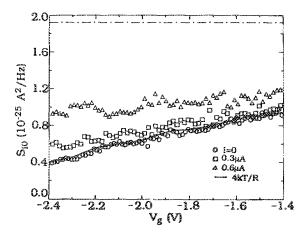
FIG. 3.  $S_{t0}$  vs  $V_g$  for I = 0, 0.3, and 0.6  $\mu$ A, where  $S_{t0}$  is obtained by fitting  $S_i = A_0 I^2 / f + S_{t0}$ . The solid curve is the Johnson noise calculated using 4kT/R. The dash-dot line indicates the theoretical full shot noise (2eI) at 0.6  $\mu$ A.
