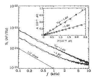
FIG. 2.  $S_i$  vs f for  $I \approx 0.43 \ \mu$ A,  $V_g = -1.6 \ V$  and  $-1.8 \ V$ . Inset shows A vs  $I^2$ , where A is obtained by fitting  $S_i = A/f + S_{i0}$ . Dash-dot lines serve as a guide to the eye. The solid line shows the  $S_i \sim 1/f$  slope.
