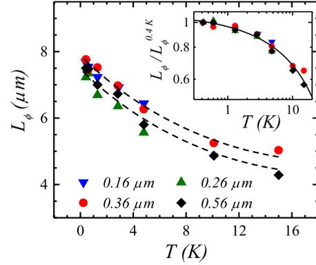
FIG. 6. (Color online)  $T$  dependence of the phase coherence length  $L_\phi$  in wires with four different widths. Dashed lines for widths of 0.36 and 0.56  $\mu\text{m}$  form guides to the eye. Inset: logarithmic plot of the  $T$  dependence of  $L_\phi$ , normalized by its value at 0.4 K, for all wires.
