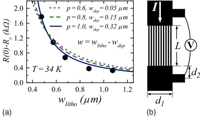
FIG. 1. (Color online) Wire set resistance  $R(B=0) - R_c$  at  $T = 34$  K as a function of lithographic design width.  $R(0)$  represents the measured resistance across the wire set and  $R_c = 114 \Omega$  the series contact resistance estimated from  $\rho_{2D}(34 \text{ K})$ . A few comparative curves calculated from Eq. (1) are depicted along with the data. Right: schematic illustration of wire set geometry. From the ratio  $d_2/d_1 \approx 0.5$  we estimate  $R_c \approx \rho_{2D}$ .
