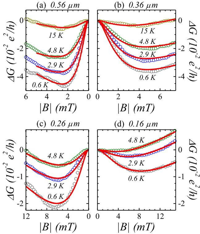
FIG. 2. (Color online) Change in conductance,  $\Delta G$ , as a function of the magnitude of the applied magnetic field,  $|B|$ , at various  $T$  for four different wire widths  $w$ : (a)  $w=0.56 \mu\text{m}$ , (b)  $w=0.36 \mu\text{m}$ , (c)  $w=0.26 \mu\text{m}$ , and (d)  $w=0.16 \mu\text{m}$ . Solid lines are fits of the magnetoconductance traces to antilocalization theory.
