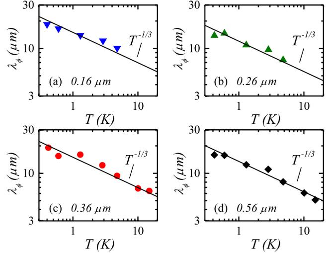
FIG. 8. (Color online) Logarithmic plot of  $\lambda_\phi$  vs  $T$  for the InSb wires of width (a)  $0.16 \mu\text{m}$ , (b)  $0.26 \mu\text{m}$ , (c)  $0.36 \mu\text{m}$ , and (d)  $0.56 \mu\text{m}$ . In all wires  $\lambda_\phi$  can be described by a  $T^{-1/3}$  law.
