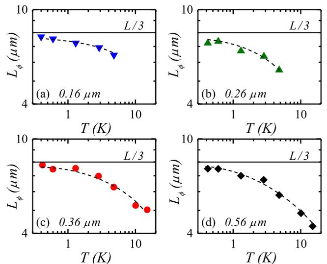
FIG. 7. (Color online) Logarithmic plot of  $L_\phi$  vs  $T$  for the InSb wires of width (a) 0.16  $\mu\text{m}$ , (b) 0.26  $\mu\text{m}$ , (c) 0.36  $\mu\text{m}$ , and (d) 0.56  $\mu\text{m}$ . Dashed lines form guides to the eye. In all wires  $L_\phi$  appears to be limited by  $L/3 = 8 \mu\text{m}$  (solid line) as  $T \rightarrow 0$ .
