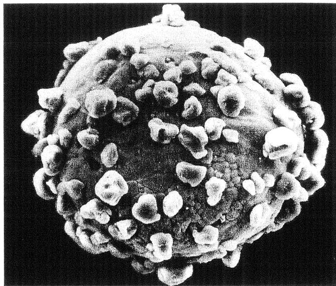
Toner particles, electrostatically attracted to a larger carrier particle.
