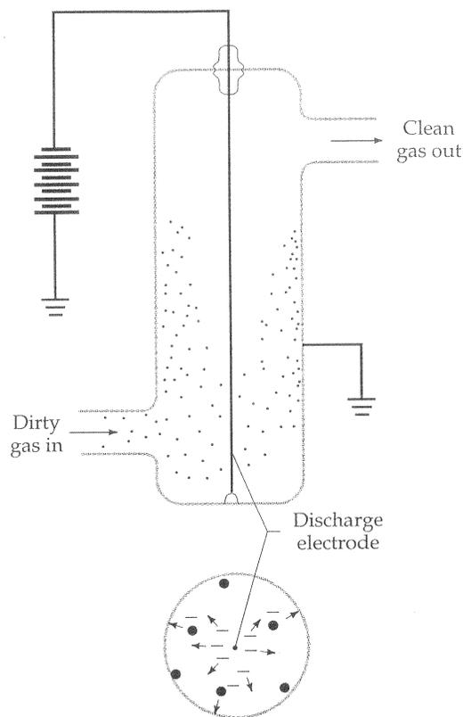
**Figure 1** Schematic diagram of the use of a corona discharge in an electrostatic precipitator.
