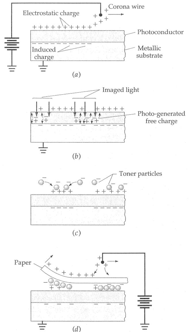
Figure 2 Steps in the xerographic process: (a) charging, (b) exposure, (c) development, and (d) transfer.
