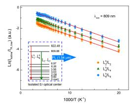
**Figure 3.** Arrhenius plots of the temperature variation of the intensity ratios of the hot lines  $L_2^h, L_4^h, L_6^h$  to that of PL lines  $L_2, L_4, L_6$ , respectively. Activation energies are found to be  $\Delta E = 13.1 \pm 0.5$  meV, equal to the spectroscopic splitting. Inset shows the Stark sub-energy level diagram of the first excited and ground states of the isolated Er optical center in GaN.
