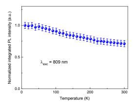
**Figure 2.** The temperature dependence of PL intensity measured under the resonant excitation ( $\lambda_{exc} = 809$  nm) indicates a low thermal quenching from  $Er^{3+}$  ions in our GaN:Er epilayer. The integrated PL intensity measurements at 1.54 µm band show a thermal quenching of 20% from 10 K to room temperature from isolated Er optical centers.
