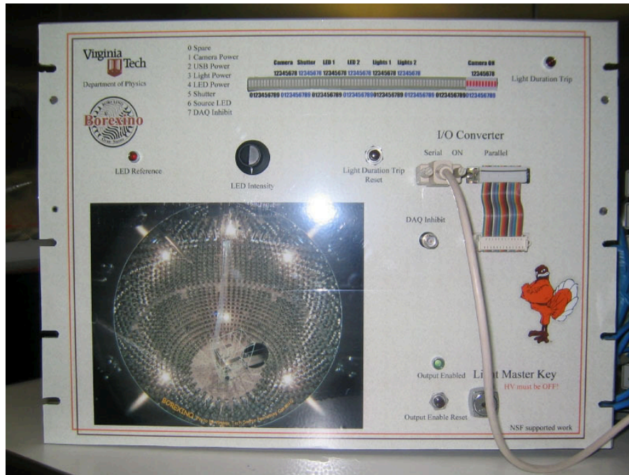
Figure 6.9: The camera control box. It is the interface between the computer and the camera system.
