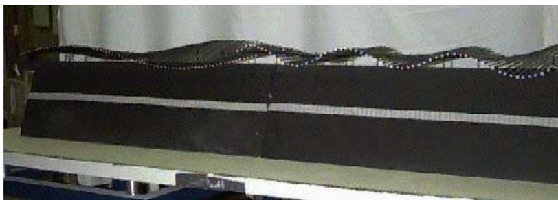
You can demonstrate: (1) wave propagation; (2) velocity in different media by two sections whose oscillators have different mass; (3) wavelength versus velocity and frequency; (4) reflection at fixed and free boundaries (by clamping the end if desired); (5) constructive and destructive interference; (6) standing waves and resonance (a mechanical oscillator for fixed known frequencies is available if desired); (7) reflection and transmission at media boundaries.
