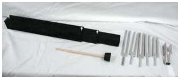
Ask students if standing waves would occur if the end were open. Most will probably think not. Demonstrate that standing waves do occur with comparable intensity. Discuss standing waves in an open pipe, calculate the resonant lengths, and demonstrate agreement.
