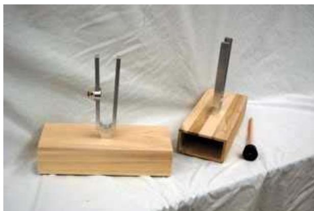
1. With the clamp remove, strike one of the tuning forks. Then stop the first tuning fork from ring and hear that the second tuning for
