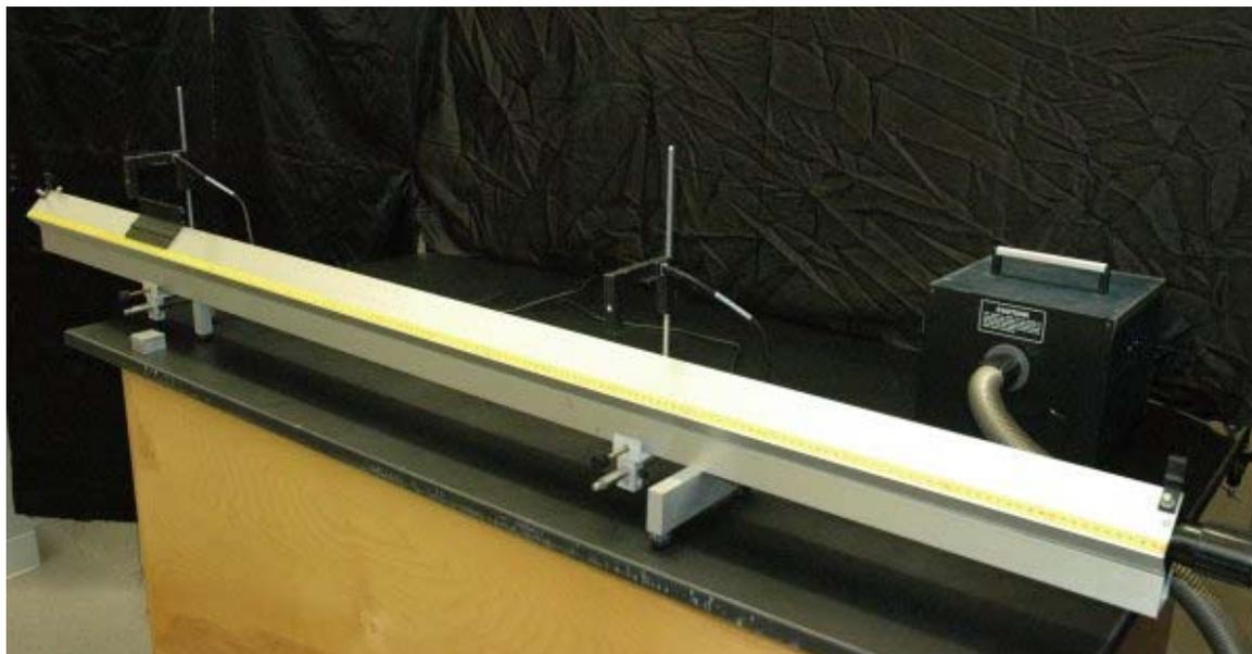
Velocity of cart is determined by dividing the length  $d$  of a light-obscuring plate by the time  $t$  that the light remains obscured ( $v=d/t$ ). The time is measured with the [Pasco 750 interface](#). These accurate determinations of velocity are then used to show acceleration.
