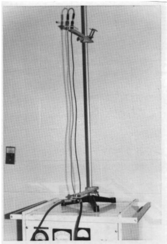
1. To demonstrate repulsion between the wires, the currents must run in opposite directions. To do this, merely remove the connector from the two binding posts on the lower end of the stand and then connect the D.C. power supply. It is important that the current be pulsed to 6 volts for only a few seconds, as a large amount of heat develops in the wires.
