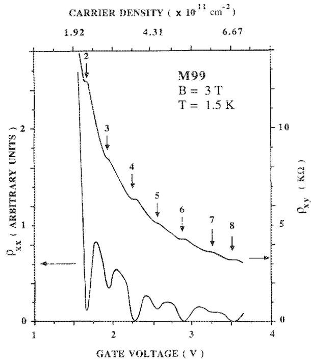
FIG. 4. Transport coefficients  $\rho_{xx}$  and  $\rho_{xy}$  for sample M99 are shown at a fixed magnetic field and as a function of the gate voltage. The vertical arrows indicate the filling factors at which the integral quantum Hall effect is observed.
