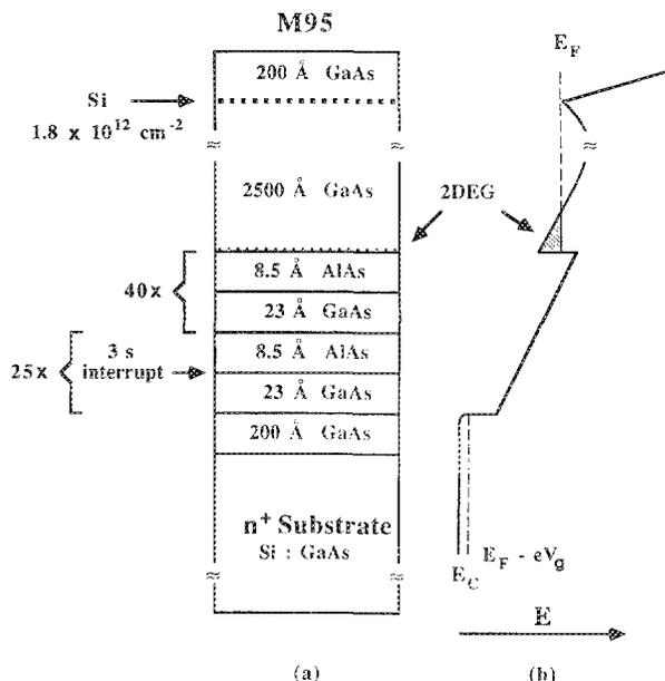
FIG. 1. Schematic description of an ISIS structure. Shown on the right is the potential diagram corresponding to the accumulation mode, achieved by applying a positive gate voltage  $V_G$  to the  $n^+$  substrate. On the left, the design structure for sample M95 is schematically shown. Note the use of a thin-layer GaAs/AlAs superlattice in place of AlGaAs barrier.
