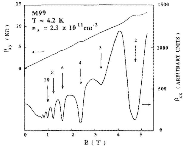
FIG. 3. Transport coefficients  $\rho_{xx}$  and  $\rho_{xy}$  for sample M99 are shown as a function of magnetic field at a fixed gate voltage. The vertical arrows indicate some of the Landau-level filling factors at which the integral quantum Hall effect is observed.
