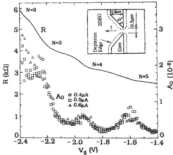
FIG. 1.  $R$  vs  $V_g$  and  $A_0$  vs  $V_g$ .  $A_0$  is obtained by fitting  $S_i = A_0 I^2 / f + S_0$  for  $I = 0.4, 0.5,$  and  $0.6 \mu\text{A}$ . The approximate plateaus in  $R$  are assigned to the quantized resistances  $h/2e^2 N$ , with  $N = 2, 3, 4,$  and  $5$ . Inset shows the device geometry (not to scale).
