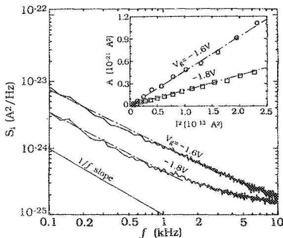
FIG. 2.  $S_i$  vs  $f$  for  $I = 0.43 \mu\text{A}$ ,  $V_g = -1.6$  V and  $-1.8$  V. Inset shows  $A$  vs  $I^2$ , where  $A$  is obtained by fitting  $S_i = A/f + S_0$ . Dash-dot lines serve as a guide to the eye. The solid line shows the  $S_i \sim 1/f$  slope.
