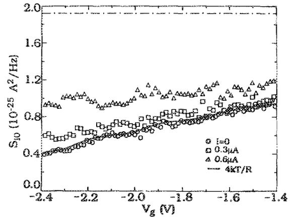
FIG. 3.  $S_{10}$  vs  $V_g$  for  $I = 0, 0.3,$  and  $0.6 \mu\text{A}$ , where  $S_{10}$  is obtained by fitting  $S_i = A_0 I^2 / f + S_0$ . The solid curve is the Johnson noise calculated using  $4kT/R$ . The dash-dot line indicates the theoretical full shot noise ( $2eI$ ) at  $0.6 \mu\text{A}$ .
