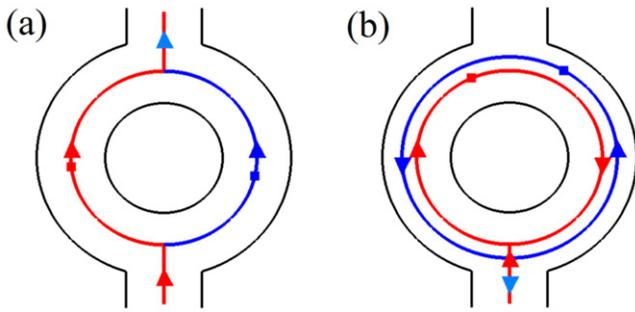
**Figure 1.** (a) Mach-Zehnder (MZ) interferometer, based on trajectories in spatially separate arms. (b) Sagnac-type (ST) interferometer, based on exact time-reversed trajectories (for clarity, trajectories are shown spatially non-overlapping).
