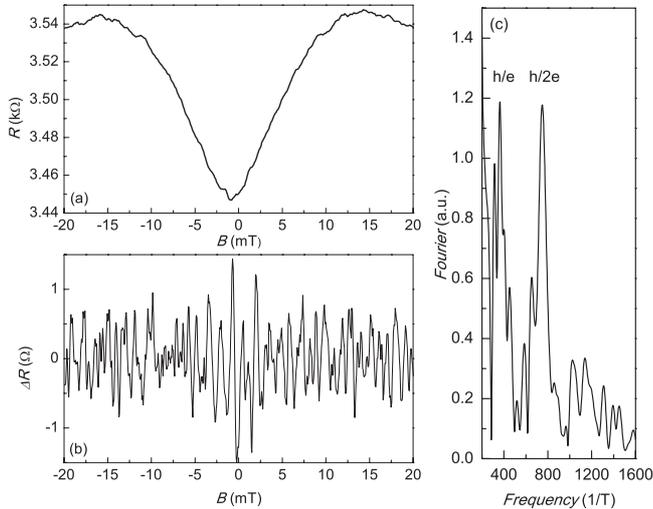
**Figure 5.** (a)  $R(B)$  versus  $B$  at low  $B$  spanning  $\pm 20$  mT; (b) After removing the WAL magnetoresistance background from (a), AAS and MZ oscillations clearly appear. (c) Fourier transform of the data in (a) with two maxima clearly marked out: the  $h/e$  maximum corresponding to MZ oscillations and the  $h/2e$  maximum corresponding to AAS oscillations.
