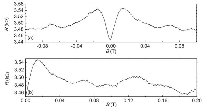
**Figure 3.**  $R(B)$  versus  $B$  measured on the array at  $T = 0.4 \text{ K}$  over two spans of 0.2 T. AAS and MZ oscillations ride on a magnetoresistance background dominated by WAL at low  $B$ . Panel (a) focuses on the region  $-0.1 \text{ T} < B < 0.1 \text{ T}$ , while panel (b) shifts to  $0 < B < 0.2 \text{ T}$  to emphasize the visibility of MZ oscillations.
