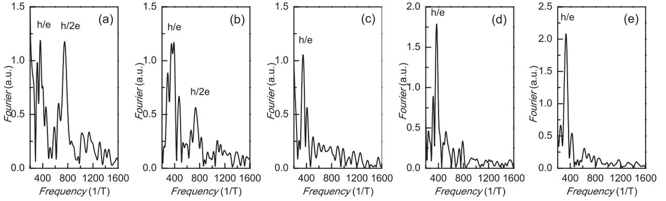
**Figure 6.** Fourier spectra illustrating the decay of AAS ( $h/2e$ ) oscillations and the survival of MZ ( $h/e$ ) oscillations with increasing  $B$ . Fourier spectra use a 40 mT span, centered at 0 mT (a), 40 mT (b), 80 mT (c), 120 mT (d) and 160 mT (e).
