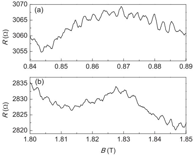
**Figure 4.**  $R(B)$  versus  $B$  over two spans of 50 mT, centered on 0.865 T (a) and 1.825 T (b). Only MZ oscillations (periodicity  $h/e$ ) are visible at these higher  $B$ .
