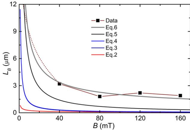
**Figure 8.** Experimental data for  $L_B$  (black squares) and calculated curves for  $L_B$  according to (bottom to top curves) equations (2)–(6) (curves for equations (3) and (4) mostly overlap for the present parameters and cannot be distinguished on the graph). The experimental data are extracted using figure 7(a) as explained in the text.
