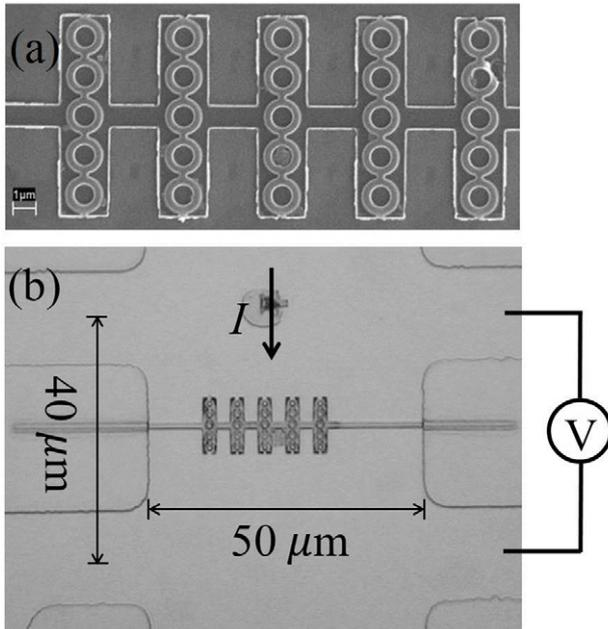
**Figure 2.** (a) Micrograph of a representative  $5 \times 5$  ring array. Each ring has average radius 650 nm and lithographic arm width 300 nm. The separation between columns is  $2.2 \mu\text{m}$ . (b) Schematic four-terminal measurement setup.
