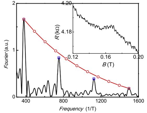
**Figure 7.** The fit to equation (1) to extract the phase coherence length  $l_\phi$  of the Aharonov–Bohm ring (data from the second sample at 0.4 K). The inset shows the Aharonov–Bohm magnetoresistance oscillations used for the Fourier transform, itself depicted as the black solid line in the main graph. The red line with open circles  $\circ$  depicts the fit to equation (1).
