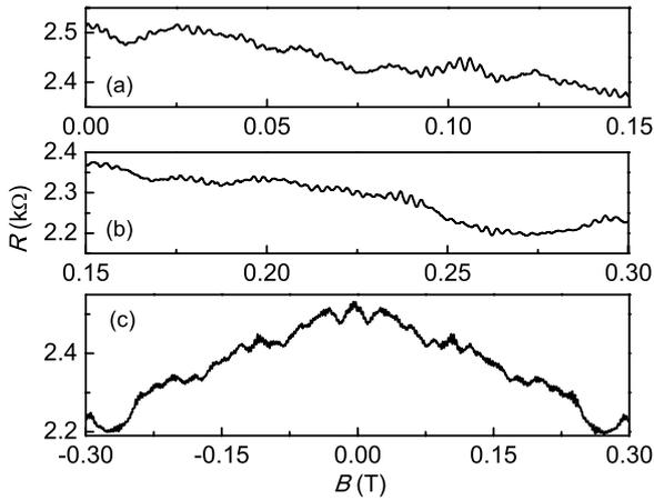
**Figure 2.** Measured Aharonov–Bohm magnetoresistance oscillations, as ring resistance  $R(B)$  versus  $B$ . Panels (a) and (b) show the ring magnetoresistance over smaller ranges of  $B$  than panel (c), which emphasizes a view of the modulation with  $B$ .
