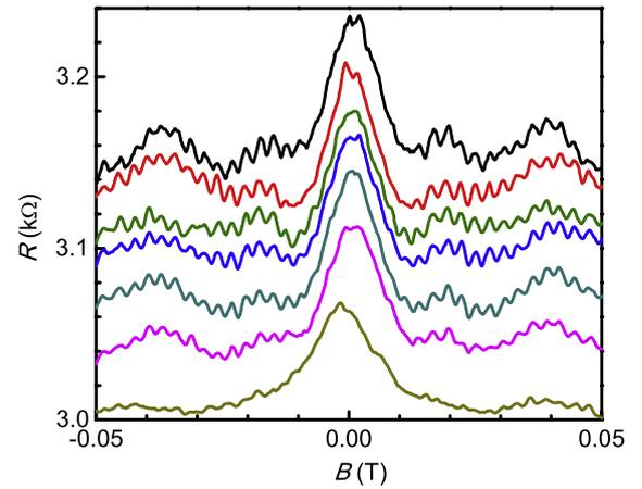
**Figure 8.** The excitation current dependence of the Aharonov–Bohm magnetoresistance oscillations at 0.4 K (data from the first sample, but with a different cooldown from that for figures 2, 3 and 6). From top to bottom, the excitation current (rms values) is 5 nA, 10 nA, 20 nA, 50 nA, 100 nA, 200 nA and 500 nA respectively. Curves are offset, actual  $R(B = 0) \approx 2.5$  kΩ.
