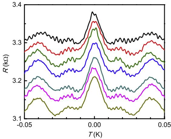
**Figure 10.** The  $T$  dependence of the Aharonov–Bohm magnetoresistance oscillations at 20 nA (data as in figure 8 from the first sample, but with a different cooldown from that for figures 2, 3 and 6). From top to bottom  $T$  is 0.4 K, 0.6 K, 0.8 K, 1.0 K, 1.2 K, 1.4 K and 1.6 K respectively. Curves are offset, actual  $R(B = 0) \approx 2.5$  k $\Omega$ .
