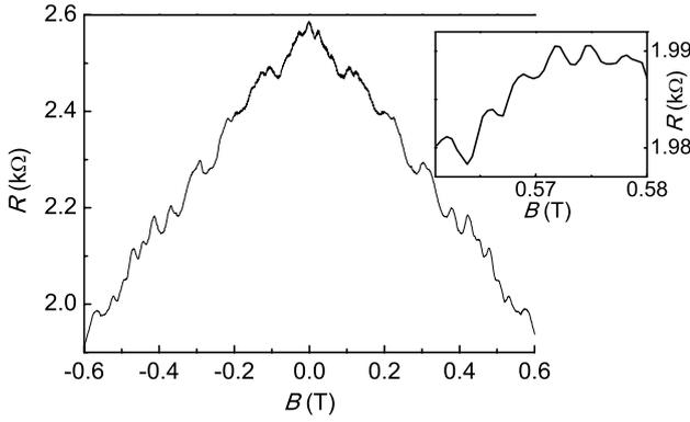
**Figure 6.** The ring magnetoresistance at 0.4 K over  $B$  from  $-0.6$  to  $0.6$  T. The Aharonov–Bohm magnetoresistance oscillations (not fully resolved on the scale of the graph) are superimposed on universal conductance fluctuations. The inset shows a selected narrow range of  $B$  around  $0.57$  T to resolve the oscillations.
