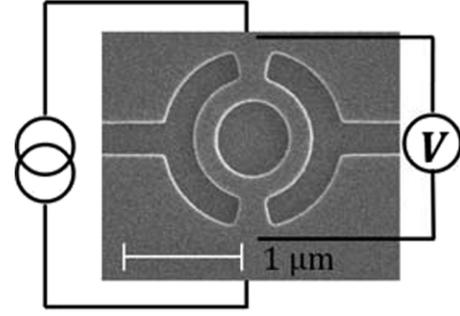
**Figure 1.** SEM micrograph of a representative Aharonov–Bohm ring, with a schematic of the four-terminal measurement setup. The darker gray areas (delineated by white borders) are etched trenches depleted of electrons, and function as barriers, forcing the electrons to travel into the lighter gray ring-shaped areas.
