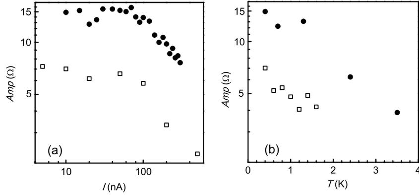
**Figure 9.** The excitation current and  $T$  dependence of the amplitude of the Aharonov–Bohm magnetoresistance oscillations (open squares  $\square$  and filled circles  $\bullet$  represent data from the first sample at different cooldowns). Panel (a) shows the excitation current dependence at 0.4 K, with a logarithmic scale on both axes. Panel (b) shows the  $T$  dependence at 20 nA, with a logarithmic scale on the vertical axis.
