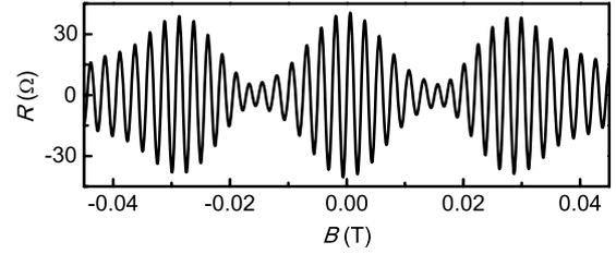
**Figure 5.** Modulation in the amplitude of Aharonov–Bohm oscillations simulated by using the three discrete frequencies deduced from the Fourier transform in figure 3(c): 376  $1/T$ , 408  $1/T$ , 447  $1/T$ , with intensities 13.2  $\Omega$ , 21.6  $\Omega$ , 5.89  $\Omega$  respectively.
