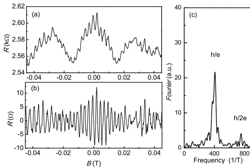
**Figure 3.** Aharonov–Bohm magnetoresistance oscillations around  $B = 0$  at 0.4 K. Panel (a) shows the raw data. Panel (b) shows the data after background removal. Panel (c) contains the Fourier transform of (b), where  $\frac{h}{e}$  and  $\frac{h}{2e}$  modes are indicated in the frequency spectrum.
