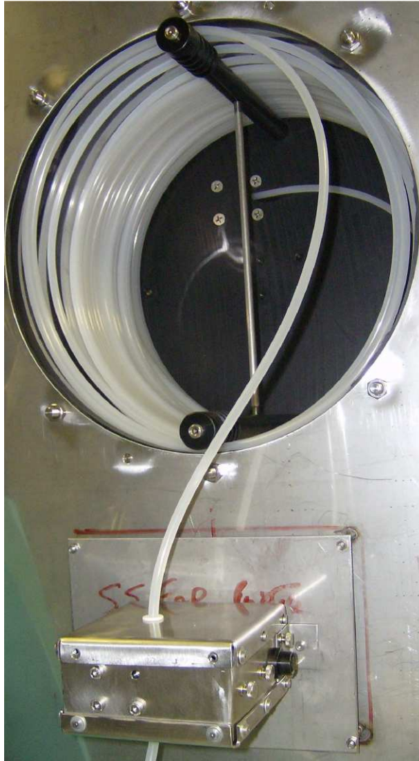
Figure 3: Tether meter housing installed below the tether storage drum. The device can be unmounted from this location and placed directly on the tube seal for an exact measurement of the length of the tether below the tube seal
