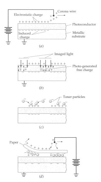
**Figure 2** Steps in the xerographic process: (*a*) charging, (*b*) exposure, (*c*) development, and (*d*) transfer.
