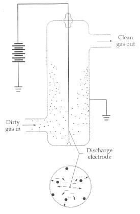
**Figure 1** Schematic diagram of the use of a corona discharge in an electrostatic precipitator.
