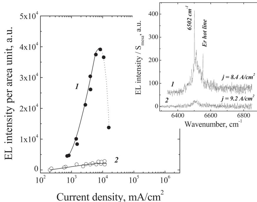
FIG. 6. Dependences of the EL intensity on the drive current density for LEDs with an active region selectively (1) and uniformly (2) doped with Er. The inset shows high-resolution EL spectra ( $\Delta\nu = 1 \text{ cm}^{-1}$ ) of these diodes taken at 80 K in the forward bias regime.
