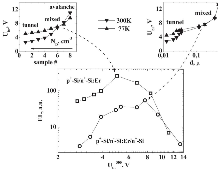
FIG. 4.  $\text{Er}^{3+}$  EL intensity as a function of  $U_{\text{br}}$  for various types of LEDs. The insets show a change of the breakdown mechanism with the carrier concentration (left) and  $n^-$ -Si:Er layer width (right).
