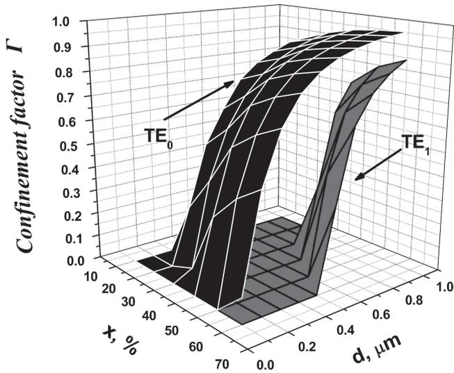
FIG. 8. Dependence of the confinement factor ( $\Gamma$ ) simulated for  $TE_{00}$  and  $TE_{01}$  optical modes in  $Si/Si_{1-x}Ge_x:Er/Si$  heterostructure on the thickness ( $d$ ) and Ge content ( $x$ ) of the  $Si_{1-x}Ge_x:Er$  layer.
