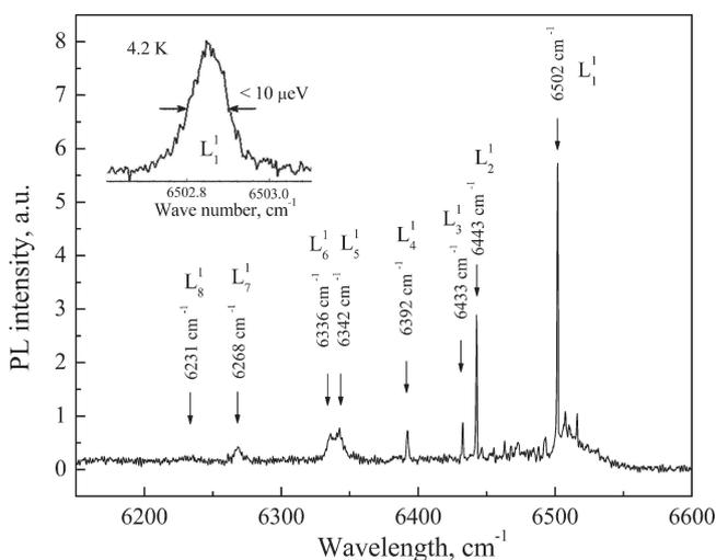
FIG. 2. PL spectrum of SMBE grown multilayer Si:Er/Si structure with predominant Er-1 center. The inset shows a high-resolution spectrum of the highest-intensity  $L_1^1$  line in the Er-1 series.
