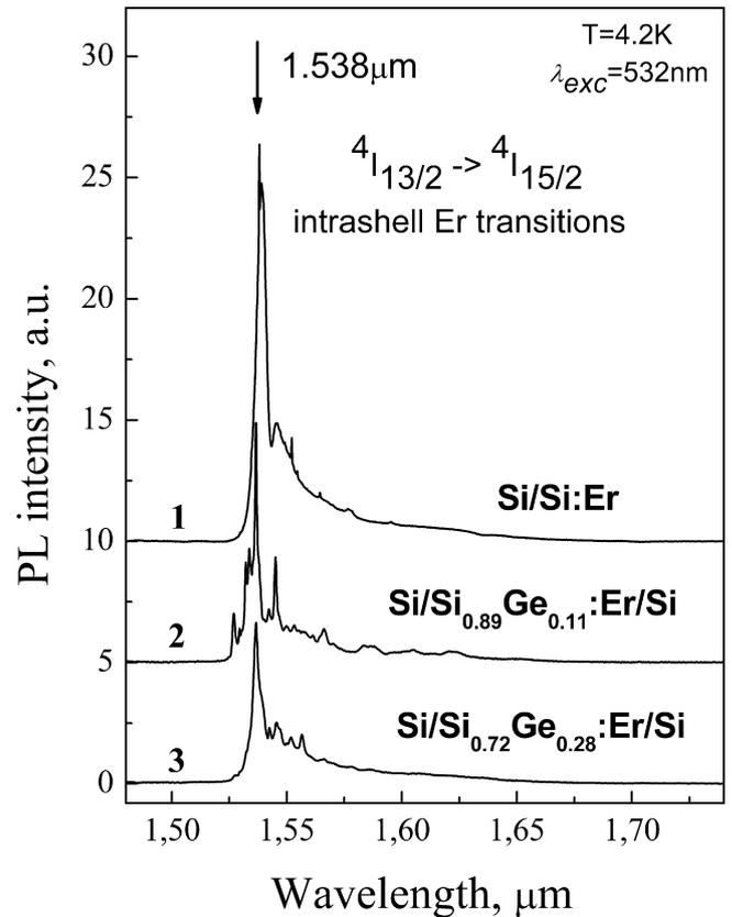
FIG. 9. PL spectra of the  $Si:Er/Si$  and  $Si/Si_{1-x}Ge_x:Er/Si$  structures. Parameters of the structures: (1)  $d_{Si:Er} = 1.8 \mu m$ ; (2)  $d_{SiGe:Er} = 0.6 \mu m$ ,  $x = 11\%$ ; (3)  $d_{SiGe:Er} = 1.1 \mu m$ ,  $x = 28\%$ .
