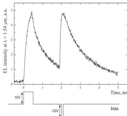
FIG. 7. Electro-optical conversion with a long-term memory effect. SEL of  $\text{Er}^{3+}$  ions has been observed a long time (up to 100 ms) after termination of the forward-bias pulse, by application of a reverse bias  $U < U_{\text{breakdown}}$  to the diode structure.
