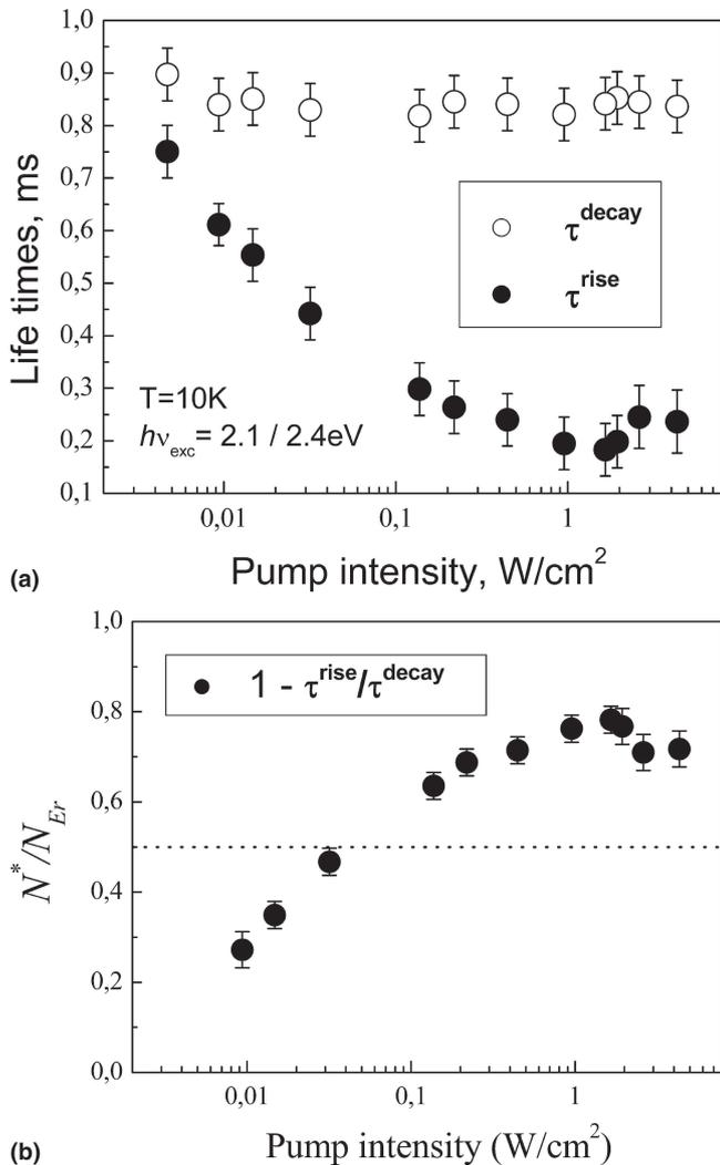
FIG. 10. (a) Life times measured for the Er-related PL peak in Si/Si<sub>0.72</sub>Ge<sub>0.28</sub>:Er/Si heterostructure, and (b) the ratio of Er ions in the excited state to the total concentration of optically active Er ions determined as a function of the excitation intensity.
