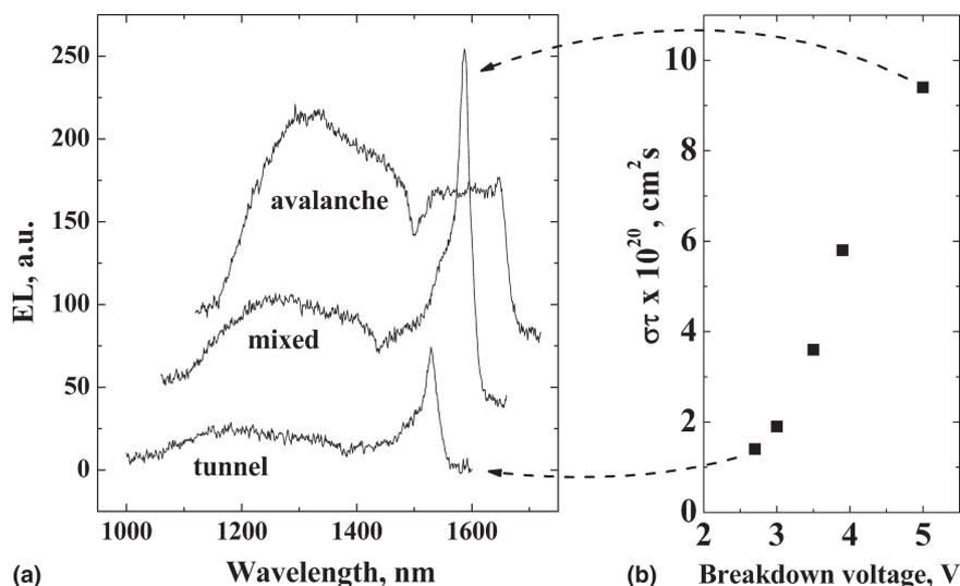
FIG. 5. (a) EL spectrum versus LED breakdown mechanism. For clearness the spectra are moved along the abscissa and ordinate axes. The spectra were taken at 300 K and drive current density of  $8 \text{ A/cm}^2$ . (b) The dependence of  $\sigma\tau$  production on the breakdown voltage.
