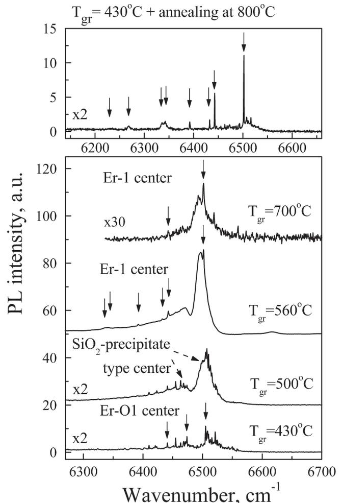
FIG. 1. PL spectra of the uniformly doped SMBE layers grown at different temperatures. The upper curve represents the spectrum of Si:Er layer grown at 430  $^{\circ}\text{C}$  after subsequent annealing at 800  $^{\circ}\text{C}$  for 30 min in hydrogen atmosphere.
