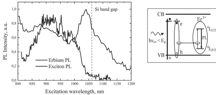
FIG. 3. Erbium- and exciton-related PL excitation spectra of SMBE Si:Er structure and a possible mechanism of sub-band-gap excitation ( $h\nu_{\text{ex}} < E_g$ ) of erbium in silicon.
