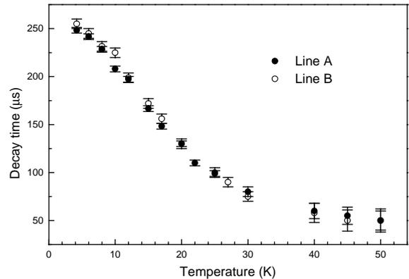
Fig. 6. The temperature dependence of decay times of A and B lines.
