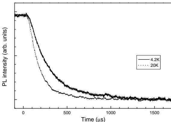
Fig. 5. Decay time for the A line of the 780 PL band measured at 4 and 20 K.
