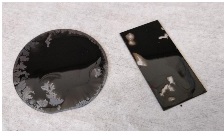
Fig. 3 Samples created by dipping a silicon wafer and a glass microscope slide into the can of Z303.
